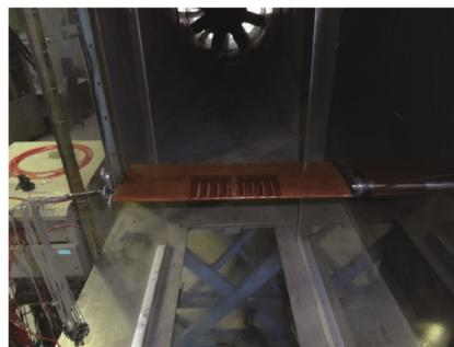
Fig. 8 Wind tunnel test section with airfoil installed inside.
