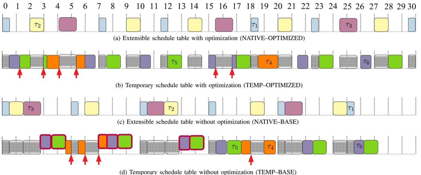
Fig. 6. Four schedule tables for an illustrative example: NATIVE-OPTIMIZED is optimized for extensibility, TEMP-OPTIMIZED has successfully added temporary tasks (hatched boxes represent native tasks), NATIVE-BASE does not consider extensibility, TEMP-BASE cannot successfully add temporary tasks, thus, some tasks (shown with red border boxes) have missed their deadlines (hatched boxes represent native tasks).
