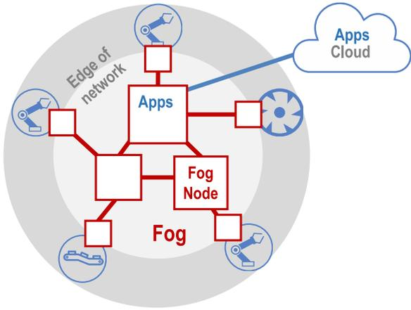
Fig. 1. Fog Computing Platform: *FNs* (boxes) are places at the edge of the network and connected via network (thick lines) to each other, equipment and the Cloud. Applications are running on *FNs* and in the Cloud.
